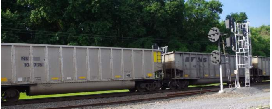
Right: Freight car America bathtub gondola. Odd thing is it is missing the NS car class
