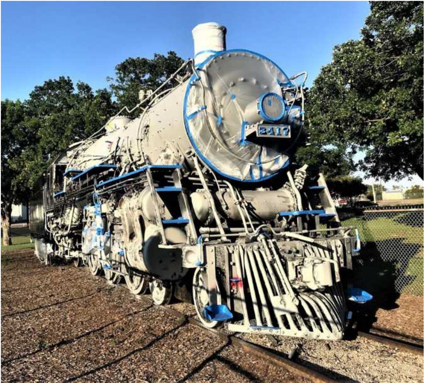
Above: AT&SF #3417 - Masked and taped. Ready for paint. May 2020. (Photo credit: Dan E Roberts.)
