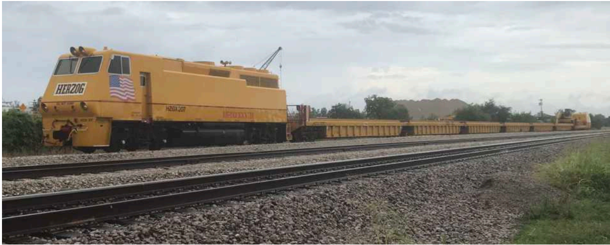
A Herzog MPM MOW (Maintenance of Way) special purpose work train is seen parked in Frisco, TX along the BNSF tracks on July 2 nd , 2021.
