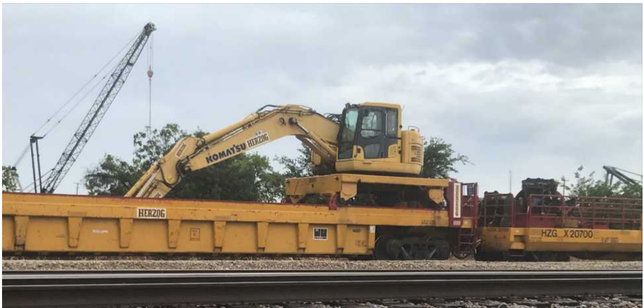
The crane pictured above, can run the entire length of the MOW Multi-Purpose Machine (MPM).
