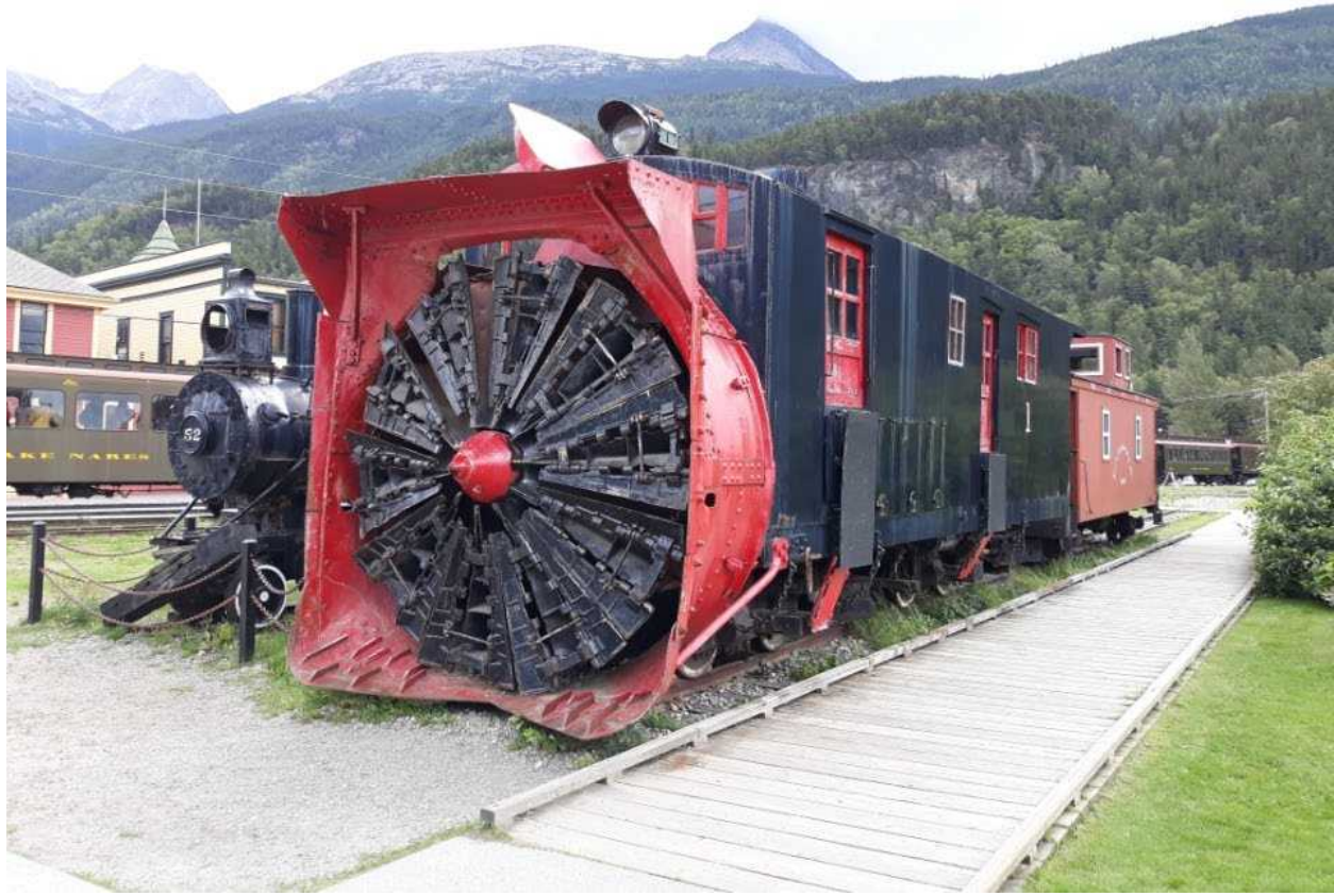
Above: Rotary Snow Plow used on the White Pass and Yukon Railroad - Skagway, Alaska. The railroad has kept one snowplow in operational condition which it uses to blow snow off the railroad in the spring before it opens for tourists.
