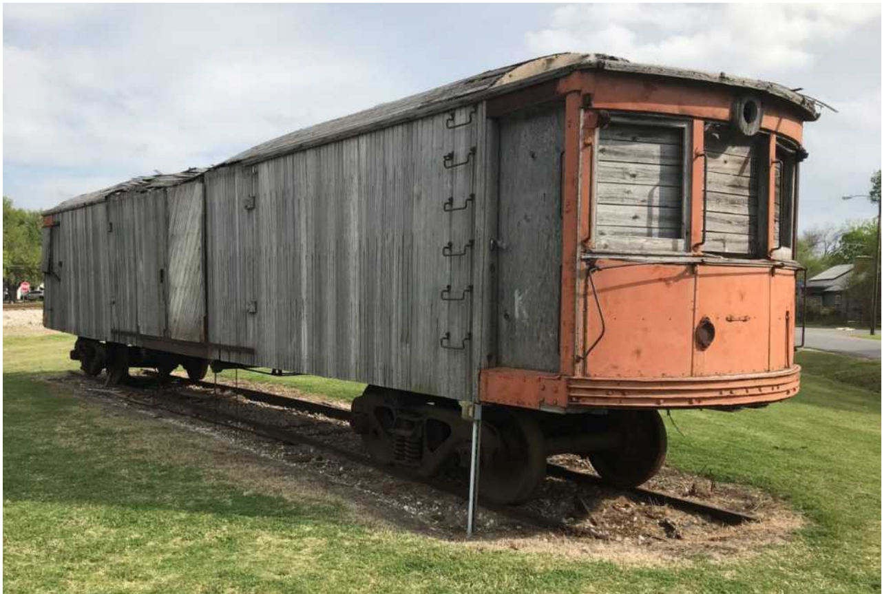
Above: Box Motor Car 501 used for freight service as seen in April 2021. The mostly wooden structure still looked like it had life in it, even though it was on life support. It should be noted that the trucks are not original to the motor car, or anywhere similar for that matter.
