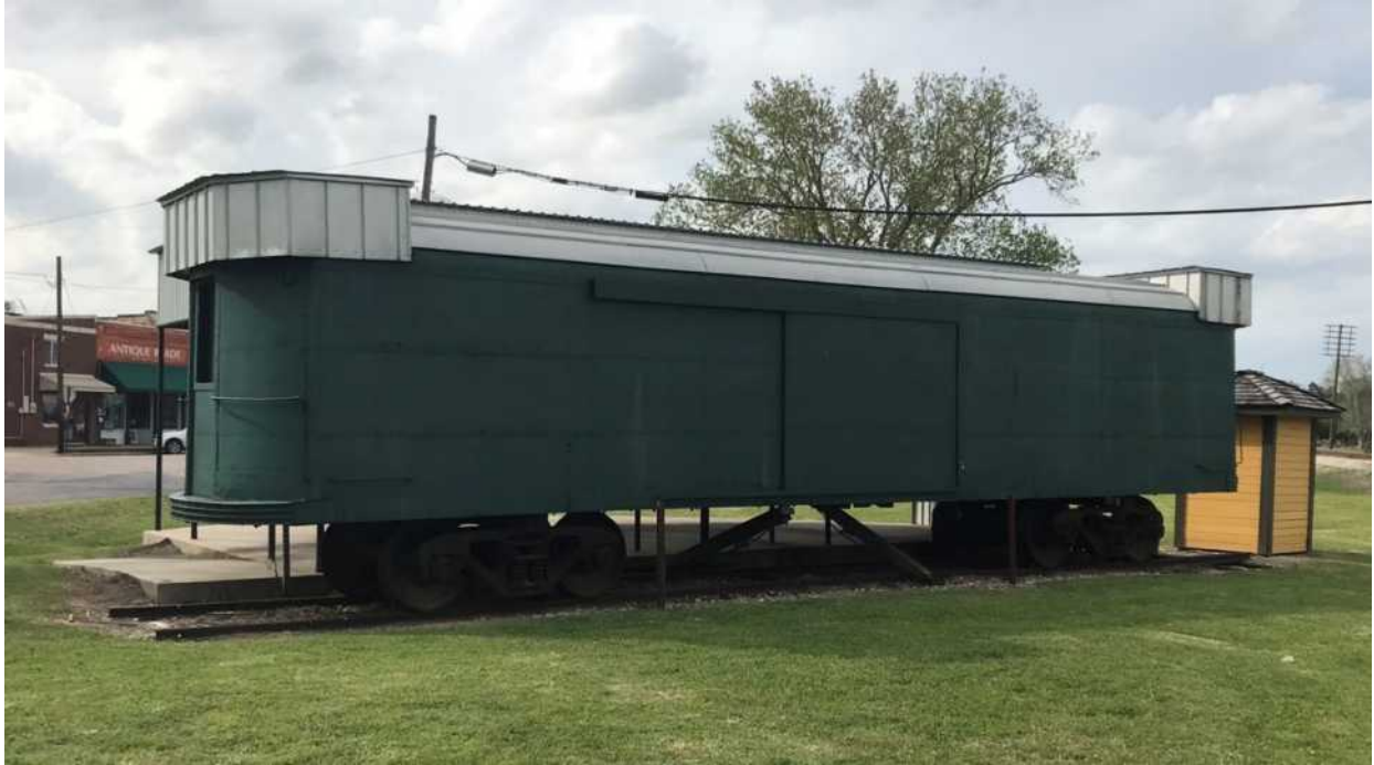
Above: Freight Trailer 608 as seen in April 2021, even though it does not have the original roof, and the roof is certainly modified. As noted on the last page, the trucks are not original to the cars. Please notice that there was actually a covered stage that was built on the other side of #608. It is now gone.
