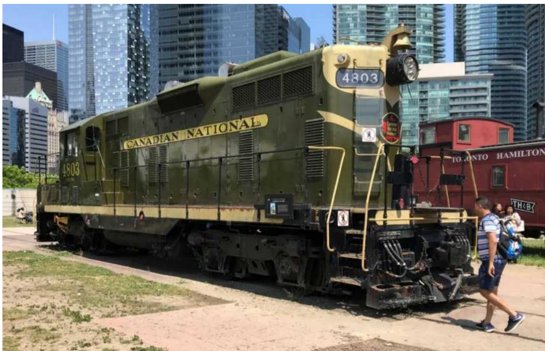
A rare high-nose GP7 built by General Motors Diesel of London, Ontario, in August, 1953, as CN 7558.
