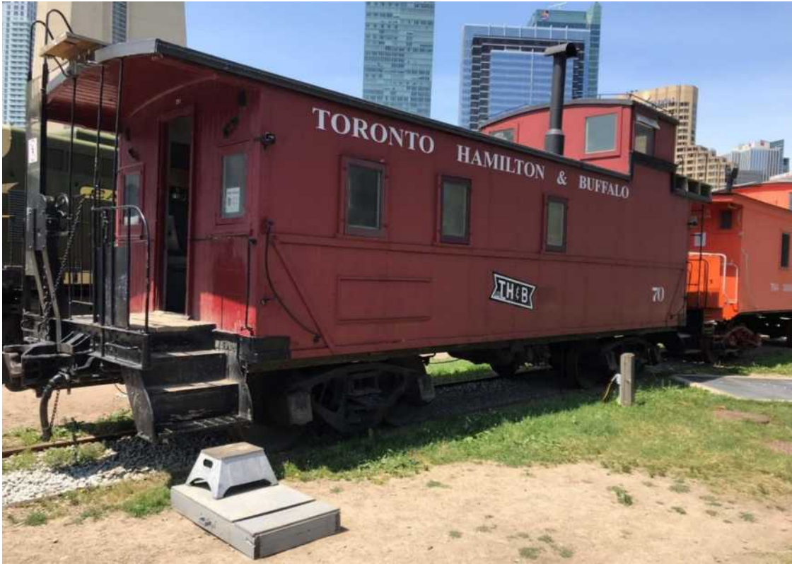
This steel-sheathed, woodside caboose was constructed in 1921 by the TH&B Railway in its Aberdeen (Hamilton) shops. Its present appearance came about in the 1950's when steel sheathing was added.
