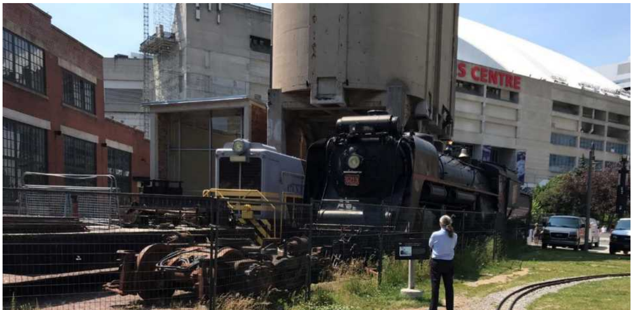
CN 6213 was built in August 1942 by the Montreal Locomotive Works. It was part of an order of 35 identical locomotives built for the Canadian National Railways during World War II. It is a U-2 class Northern-type steam locomotive with a 4-8-4 wheel arrangement and was used to haul both passenger and freight trains. The 6213 is seen above in the maintenance facility, as it gets on-going maintenance.
