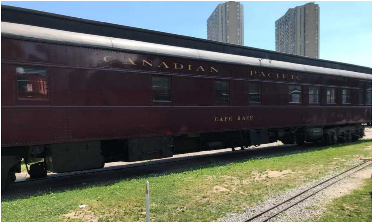
Cape Race was built for the Canadian Pacific Railway in 1929 as the River Liard . The car was one of a series of 15 River cars fabricated at National Steel Car in Hamilton. Cape Race was converted to Business Car 13 in 1963 and used by the CP superintendent based in Kenora, Ontario.
