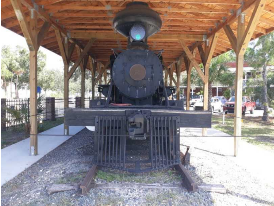
“Old Cabbage Head” gets its name from the shape of its smoke stack. Because it has a wood burning boiler, a bulbous smoke stack was needed to catch burning embers that flew out of the engine.
