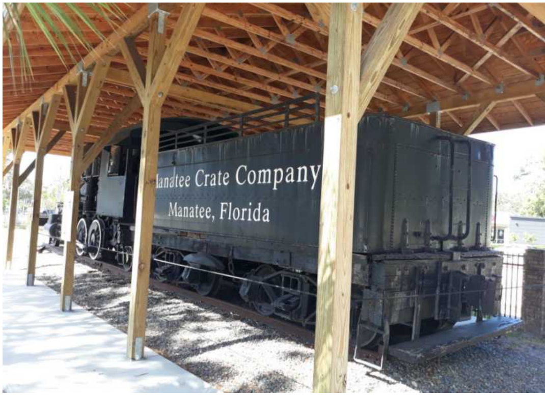
“Old Cabbage Head” was a wood burning locomotive and the tender was used to store the logs for fuel.
