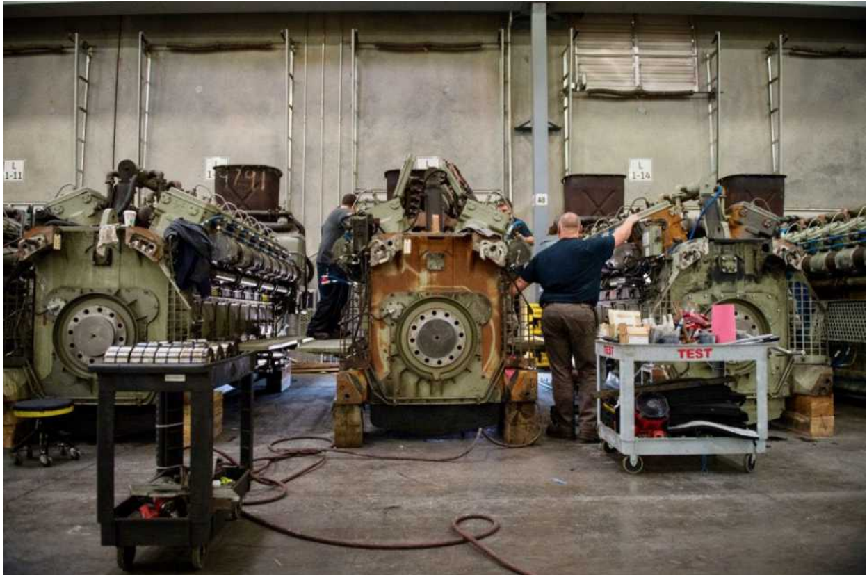
Above: GE’s huge locomotive factory outside Fort Worth, Texas, is filled with locomotives in various states of assembly. Here’s the engines section. Images credit: GE Transportation.
