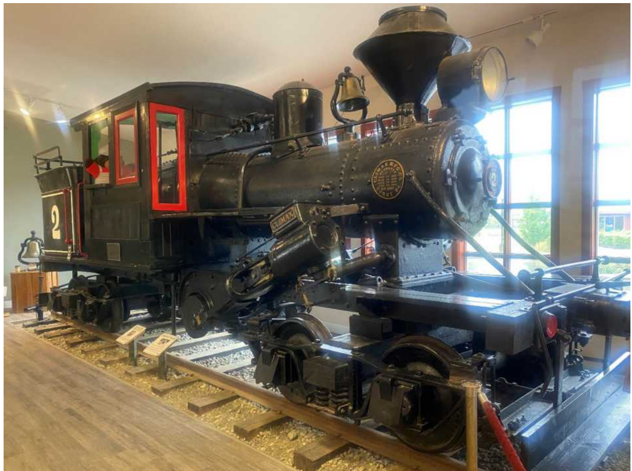
Another locomotive in the museum’s collection is this Shawnigan Lake Lumber Co. No. 2 Climax Locomotive (1910 – 23 ton Class “B” Climax locomotive).
