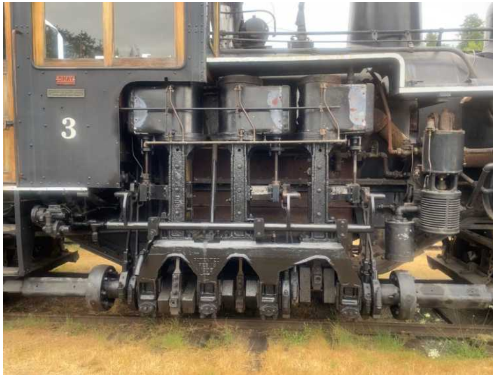
Shay locomotives have a fascinating system of gears that give the locomotive ultimate power to transverse steep inclines for logging and mining related railroads. The Shay is built for power, not for speed. Climax locomotives are also built specifically for power and not speed.
