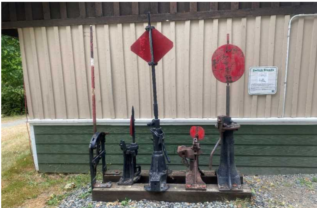
A display of some commonly used Switch Stands used in British Columbia.
