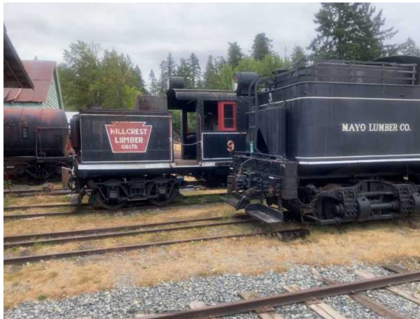
Also, the collection includes Hillcrest Lumber Co. No. 9, a 1915 – 45-50 ton Class “B” Climax locomotive, one of very few Climax engines in the world that are in operational condition; and Mayo Lumber Company No. 3, a 1924 Shay locomotive that operated in Vancouver Island’s forest industry.
