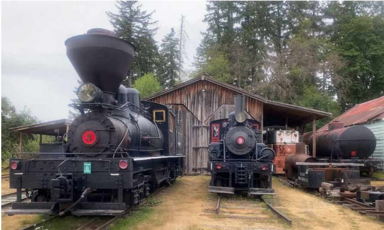
Here is a front end view of Shay No. 3 and Climax No. 9. In the right side of the picture is the unusual British Columbia Forest Products No. 9 80-DE-7-B locomotive built by The Whitcomb Locomotive Co. (80-ton, 0-4-4-0, Double Power Plant Diesel Electric). It was originally built for the US Navy in 1943.
