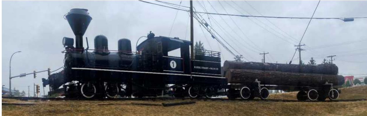
As visitors approach the entrance to the museum, they are greeted with this Bloedel Stewart & Welch No. 1 shay locomotive (1911 – 42 ton Class “B” 2-truck Shay locomotive built by Lima Locomotive Works in Ohio). It may not be obvious, but it was pouring down rain when this picture was taken.
