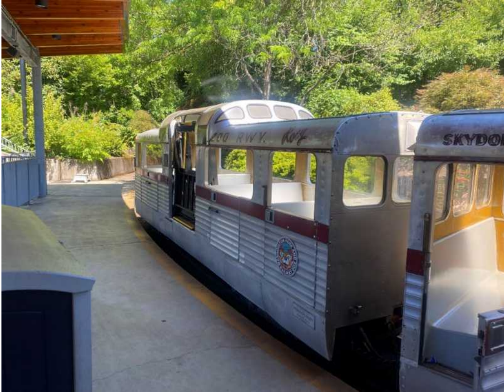
The rear car had a dome and also contained a wheelchair lift as seen in the middle of the car.
