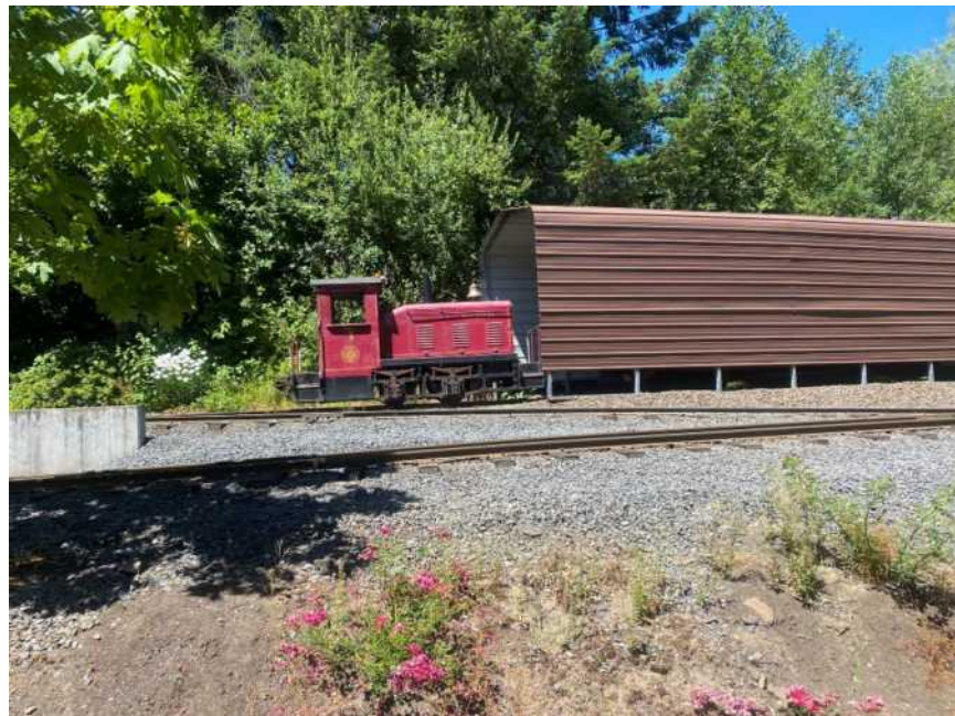
The Washington Park & Zoo Railway also possess a couple of small industrial diesel locomotives used for track maintenance and switching.
