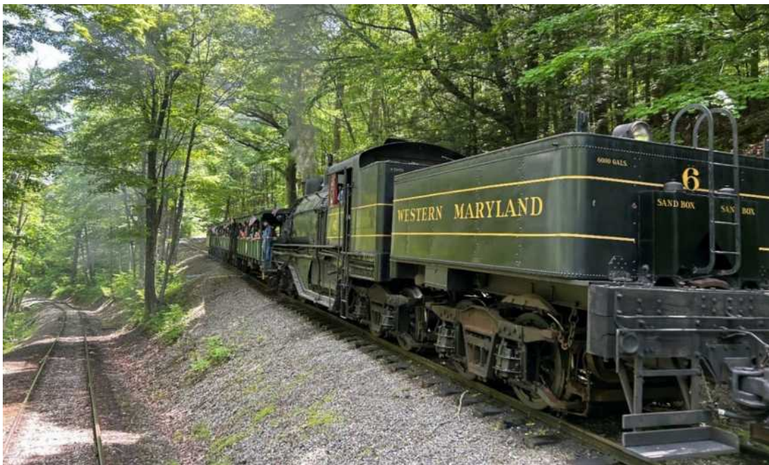
Shay #6 (the largest one made) was built for Western Maryland RR and is seen on a switchback on its way to Whittaker Station. The complete route to Bald Knob (altitude +4800 ft.) includes grades up to 13% and two switchbacks.
