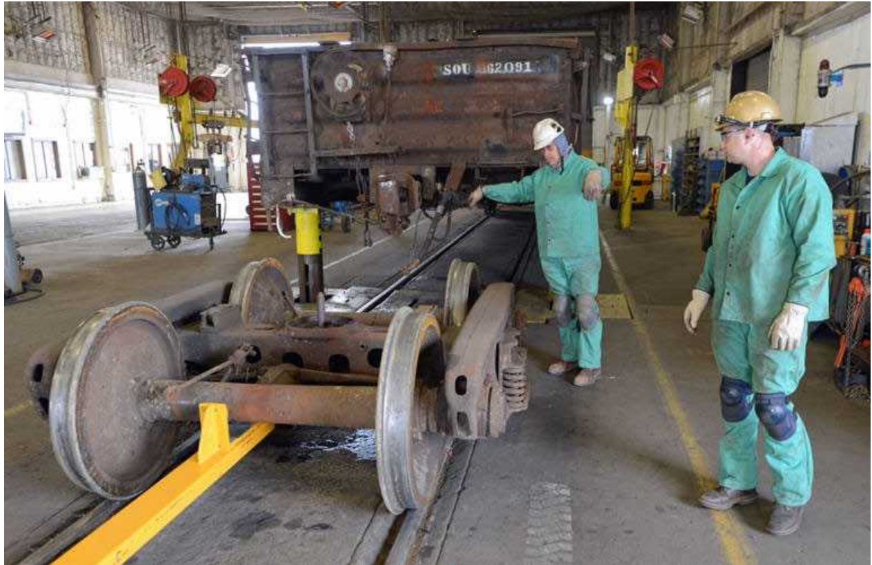
Norfolk Southern carmen roll a truck with bad wheels out from beneath a steel gondola in the Luther Yard shops in North St. Louis, Missouri, in March 2013. Steve Smedley. Provided by Trains.com
