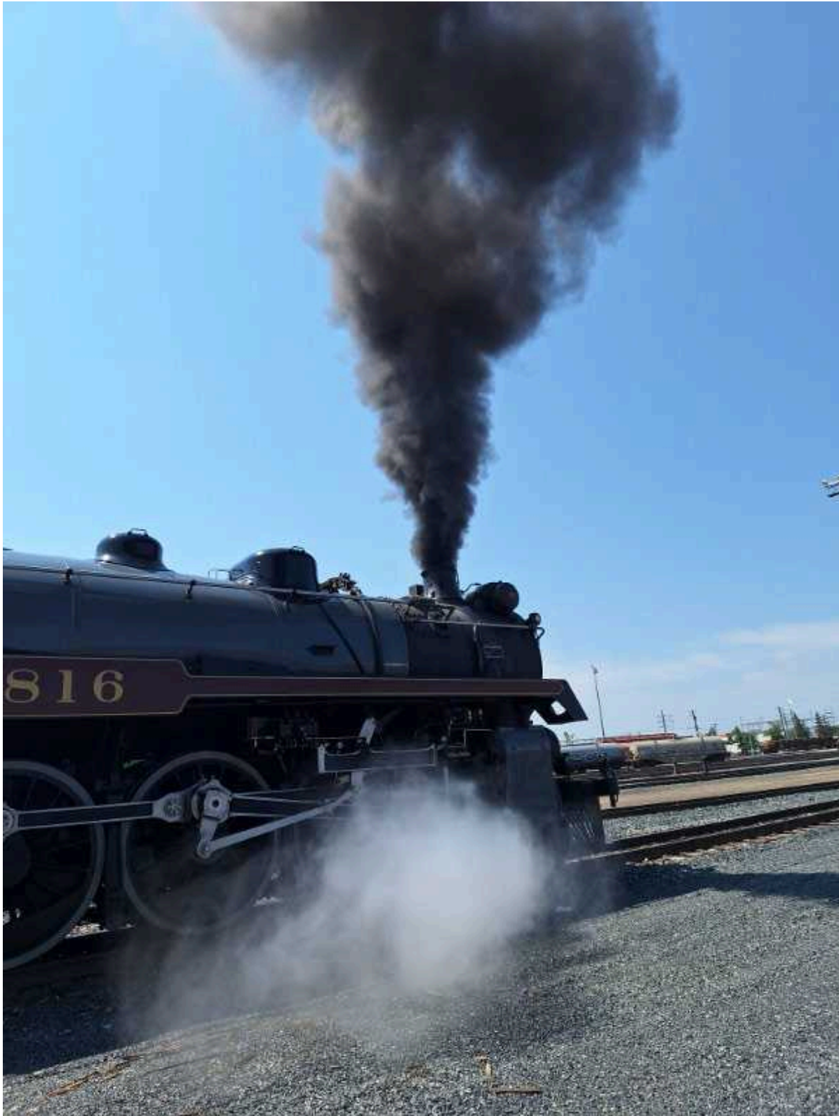
Canadian Pacific 2816, also known as the " Empress ", is seen showing off for the crowd. She is a preserved class "H1b" 4-6-4 Hudson-type steam locomotive built by the Montreal Locomotive Works in December 1930 for the Canadian Pacific Railway. It is the only non-streamlined H1 Hudson to be preserved.
