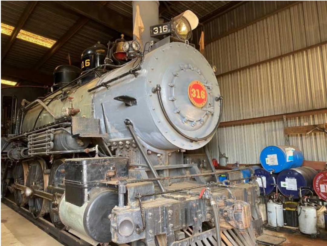
Former Texas and Pacific Railway #316, 4-6-0 built by A. L. Cooke.
