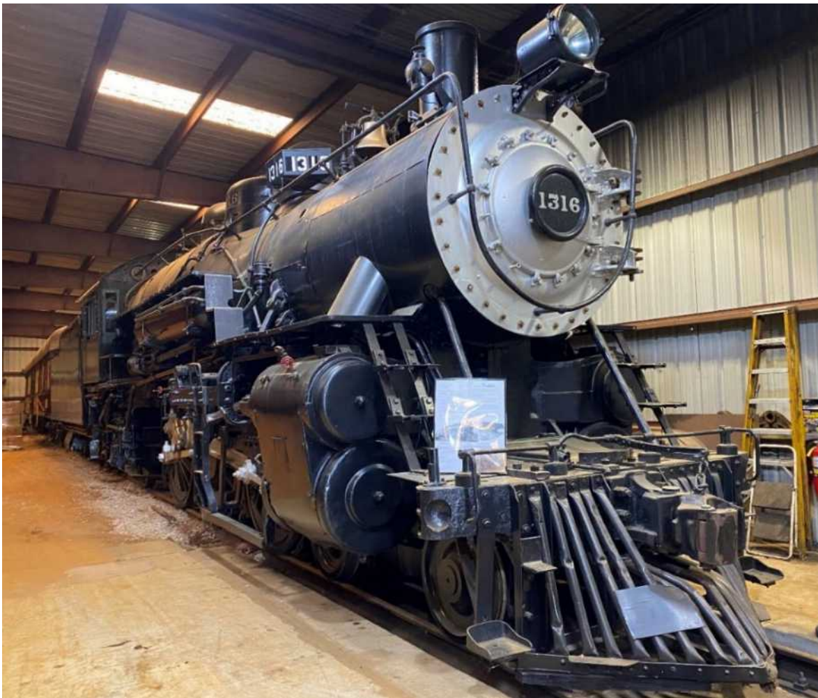
Former Santa Fe #1316, 4-6-2 built by Baldwin Locomotive Works. Photo by Linda Swan.
