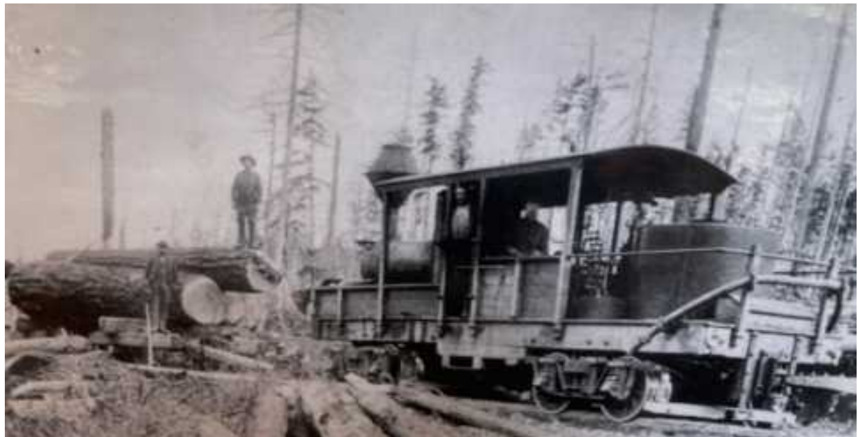
This picture was displayed at the British Columbia Forest Discovery Centre and is a perfect example of a Pole Railroad . Wood poles were plentiful but steel rails cost money. At the turn of the century, three primitive wooden railroads operated in the Cowichan district on Vancouver Island. If you look close, you can see unique wheels on the locomotive made especially to ride over log poles.
