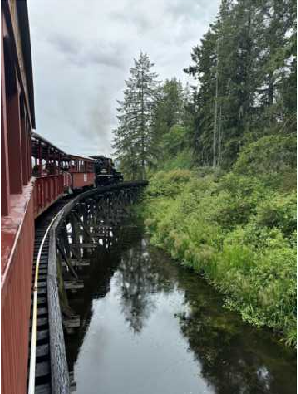
Hillcrest Lumber Company steam locomotive #1 (24-ton, 2-truck, 36" gauge Shay) pulls visitors over the Somenos Lake Trestle at the BC Forest Discovery Centre in Duncan, British Columbia after its restoration.
